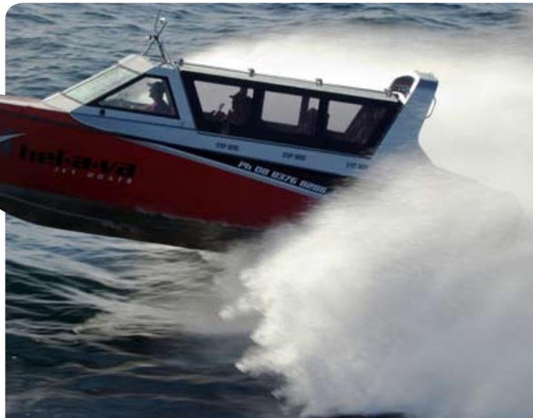
Beneath us, a pair of 5.9-litre turbo-charged engines, capable of pushing out over 1,200 litres of water per second, power us ahead with so much thrust that our safety harnesses start to strain”
